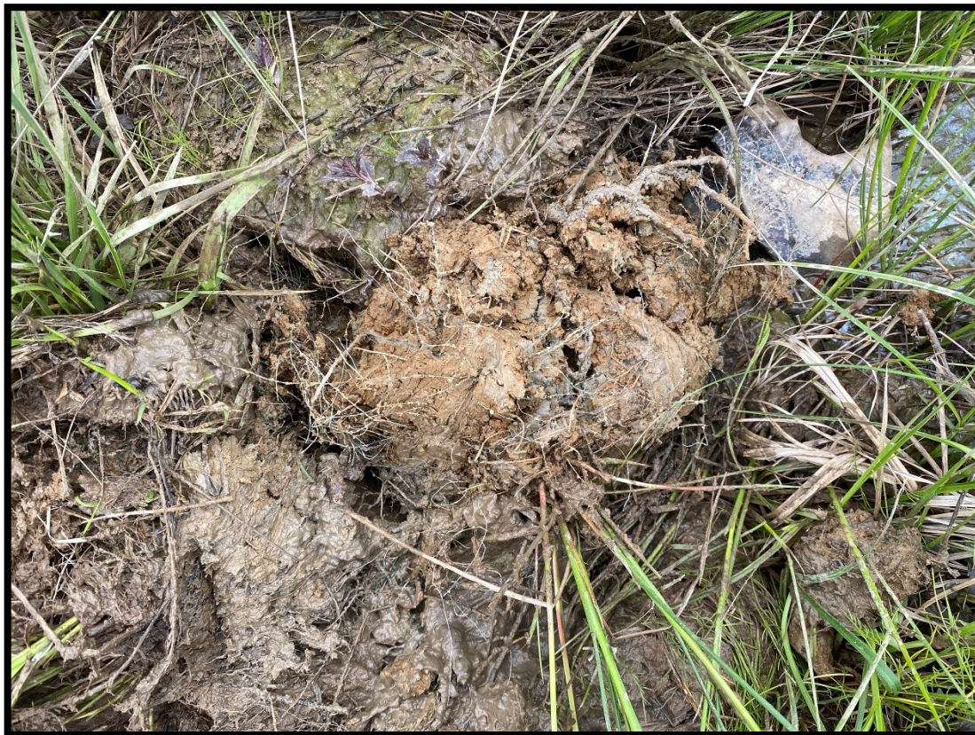
Photo 4: View of WTP-28. Soil matrix 10YR 4/2 with 10YR 5/1 redox concentrations.
