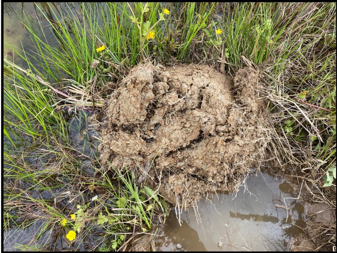
Photo 41: View of WTP-29. Soil matrix 10YR 5/1 with 7.5YR 5/6 redox concentrations.
