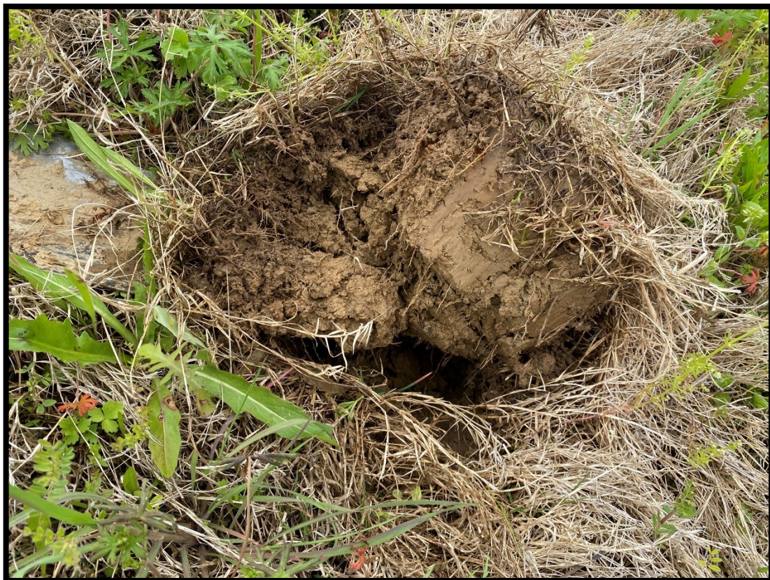
Photo 42: View of UTP-29. Soil matrix 10YR 4/6 with no redox concentrations.
